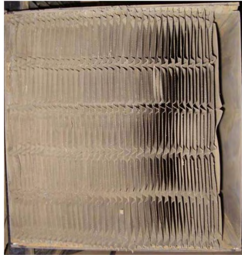
Competitor Plate Catalyst from Different Unit for Illustration (3 Spacers/Plate)
